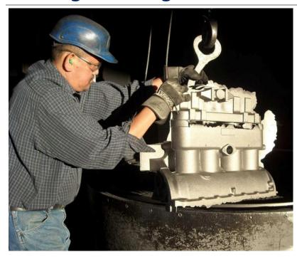
Long time MAFCA member **Terry Burtz** of Campbell California has long been working on a project to have a new Model A engine block, crankshaft and connecting rods manufactured. The engine will be identical to the original Model A engine on the outside but will have 5 main bearings, a balanced crankshaft, and full pressurized oil system.
